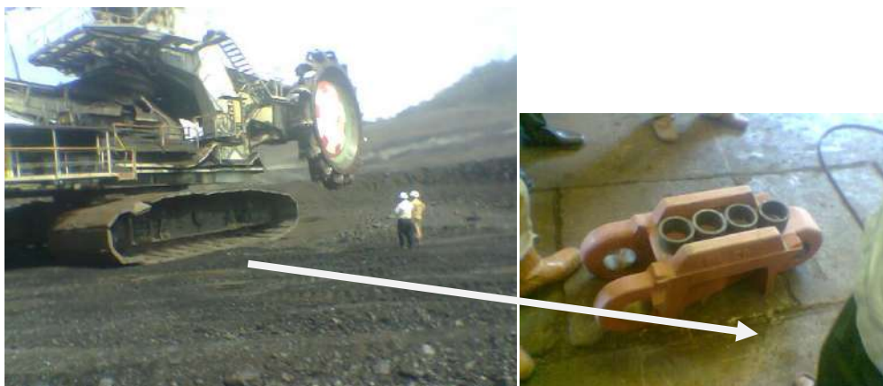
Gambar 1. Bucket Wheel Escavator dan Spare Part Link Track
